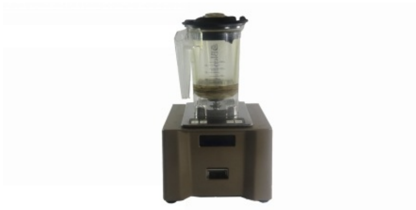
Industrial blender and accessory jar used for grinding beans and grains into flower. The smaller jar is more suitable for grinding herbs.
